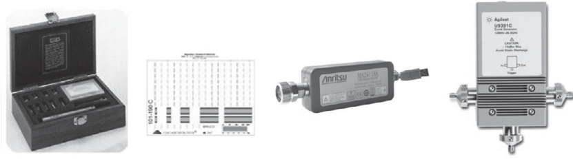
Figure 2.54 Calibration elements for NVNA measurements: from left to right, calibration box, on-wafer calibration substrate, power sensor, and harmonic phase reference. Images © external vendors.
