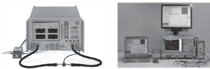
Figure 2.52 Two mixer-based NVNAs. Images © external vendors.
